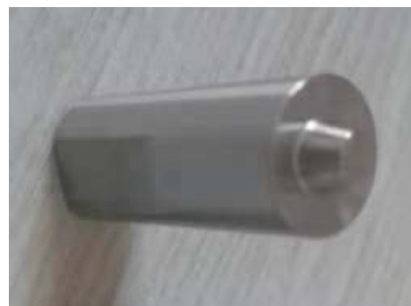
图 2 试验采用的搅拌头外形示意 Fig. 2 Outline diagram of mixing head used in the test
