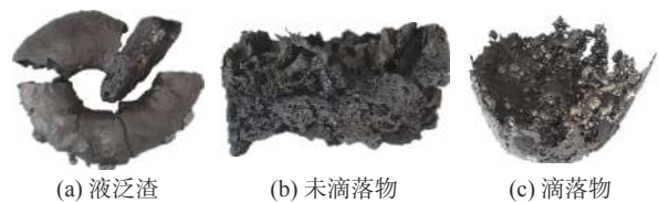
图 2 钒钛烧结矿软熔性能测定后的试样 Fig. 2 Different samples of vanadium-titanium sinter after softening-melting property testing
