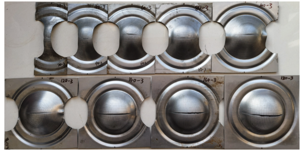
图 5 成形极限曲线测试结束后试样 Fig. 5 Specimens after the forming limit curve testing
