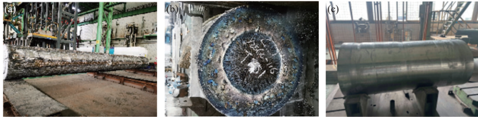
(a) 电极; (b) 铸锭; (c) 扒皮后光锭
