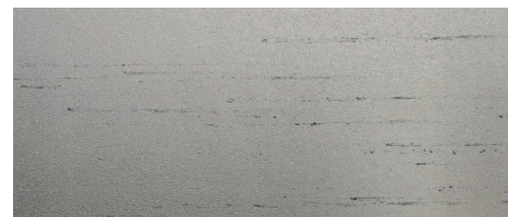
图5 TA2 热轧酸洗卷表面起皮宏观形貌 Fig. 5 Macro morphology of peeling on surface of TA2 hot-rolled pickled coil
